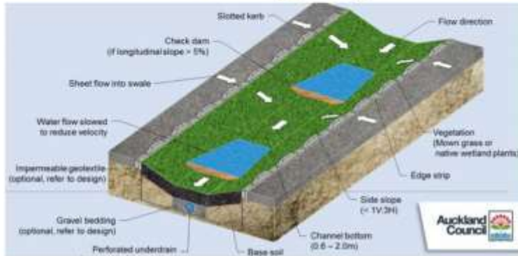
Figure: Cross-sections of a swale (Auckland Council draft)
