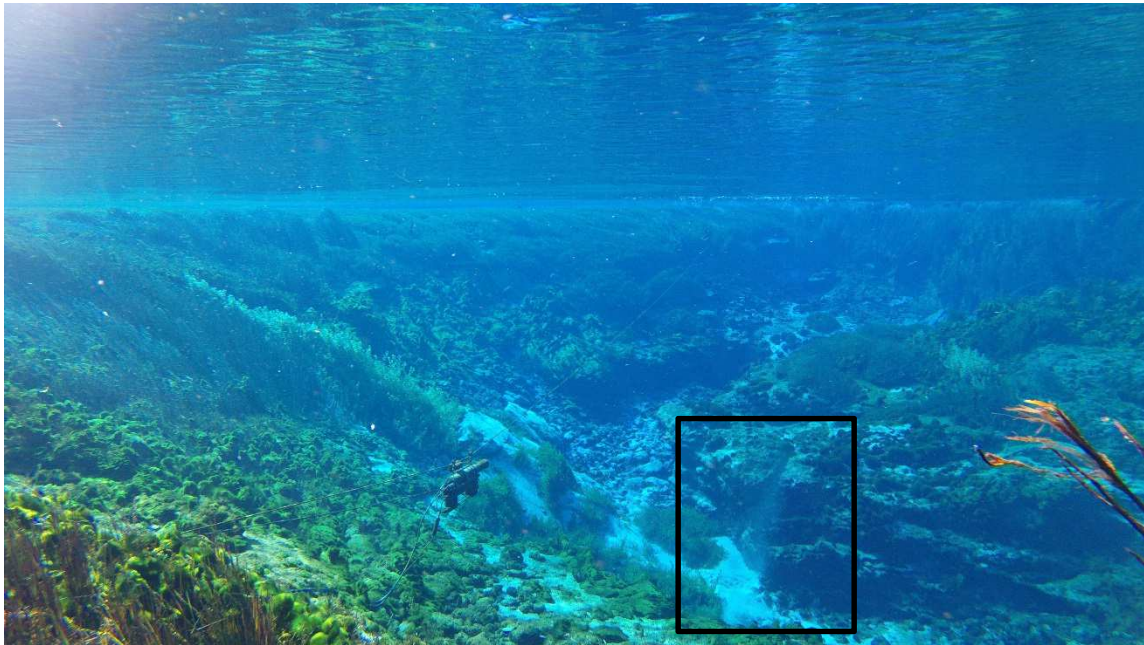
Figure 4-1: Deployed instrumentation in Te Waikoropupū Springs. The instrument hangs suspended about 1 m off a sloping bathymetry near the springs deepest basin. Note: The ‘jet’ (blur) of white sands (black box), and white sands scattered around the basin area.
