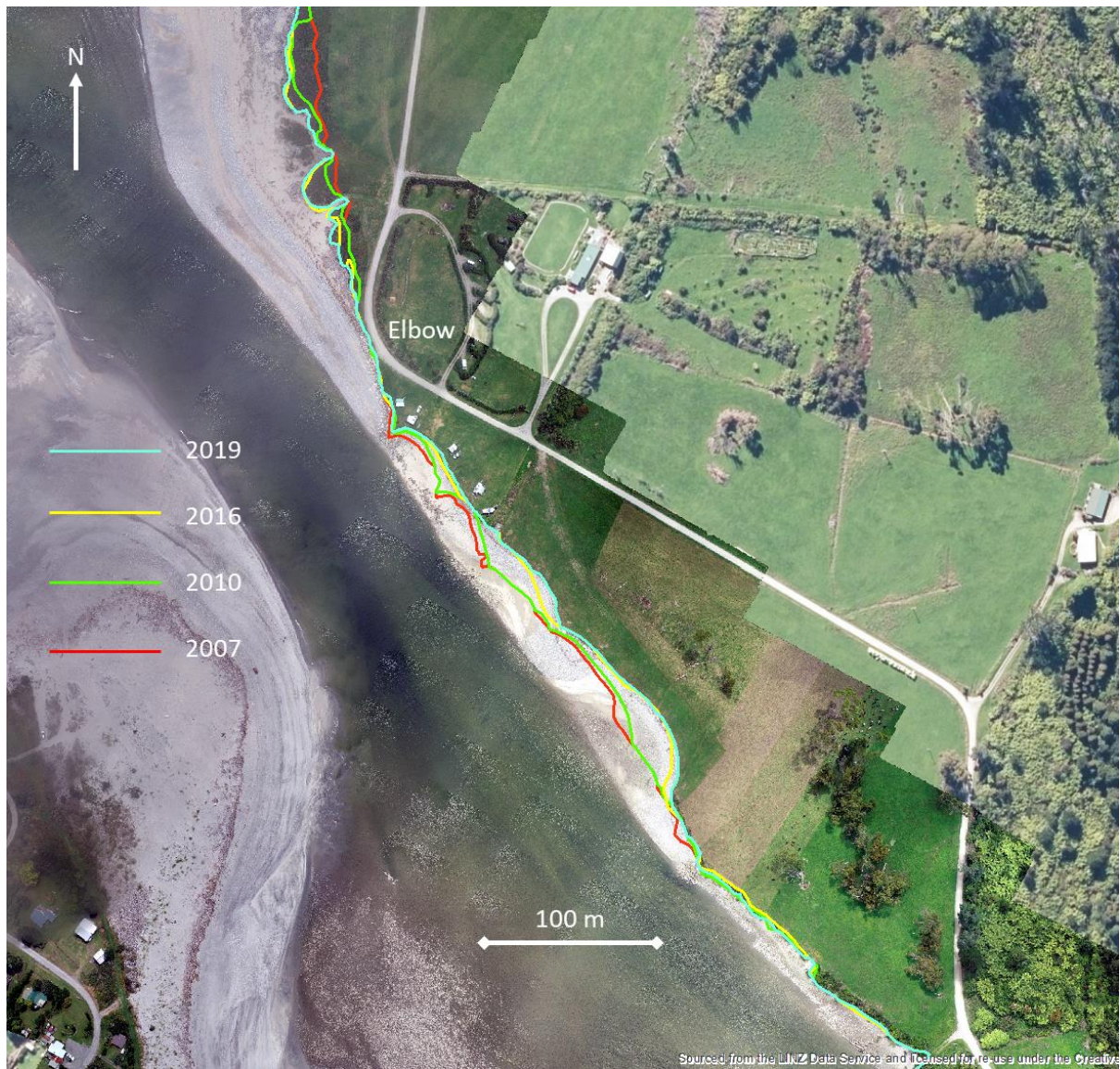
Figure 4-2: North bank locations between 2007 and 2019 overlaid on 2019 imagery. Bank/shore edge positions mapped off edge of vegetation on georeferenced imagery.
