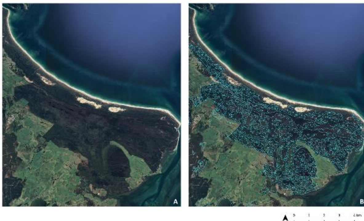
Figure 15: A. Wetland area near Kaimaumau, Northland. B. an example of a 20-cluster segmentation based on bands 4, 3, 2 and 8. Different classes correspond to different vegetation patterns suggesting hydrological or successional controls over vegetative cover.
