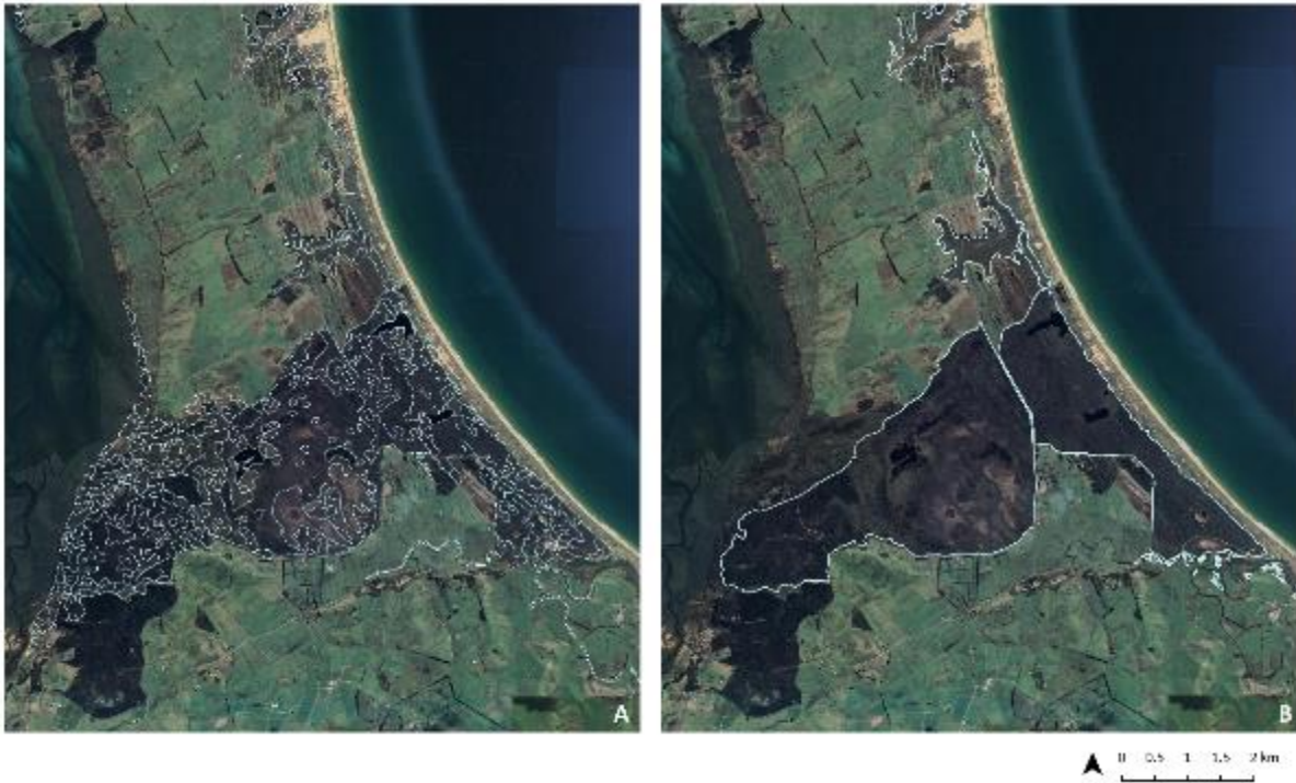
Figure 18: Wetlands north of Ohia, A is the OBIS analysis grouping areas that have a similar spectral signature, this is consistent with changes in vegetation. B shows the outline of the currently mapped wetland extent for comparison.
