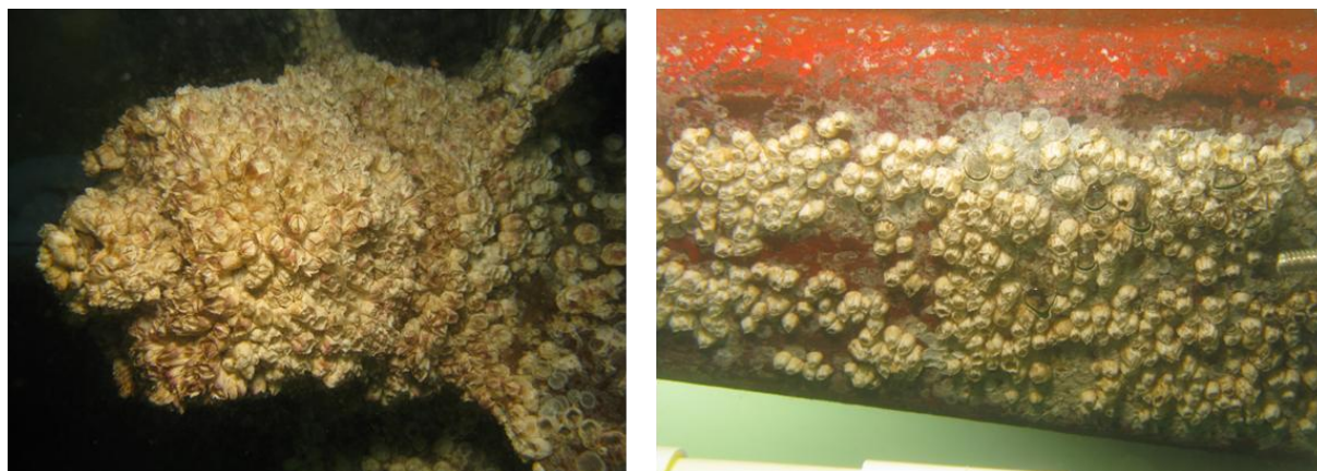
Figure 3. Examples of high percentage cover of boat niche areas (LOF 5 for a propeller and keel bottom) with an apparent taxon richness of one (barnacles).
