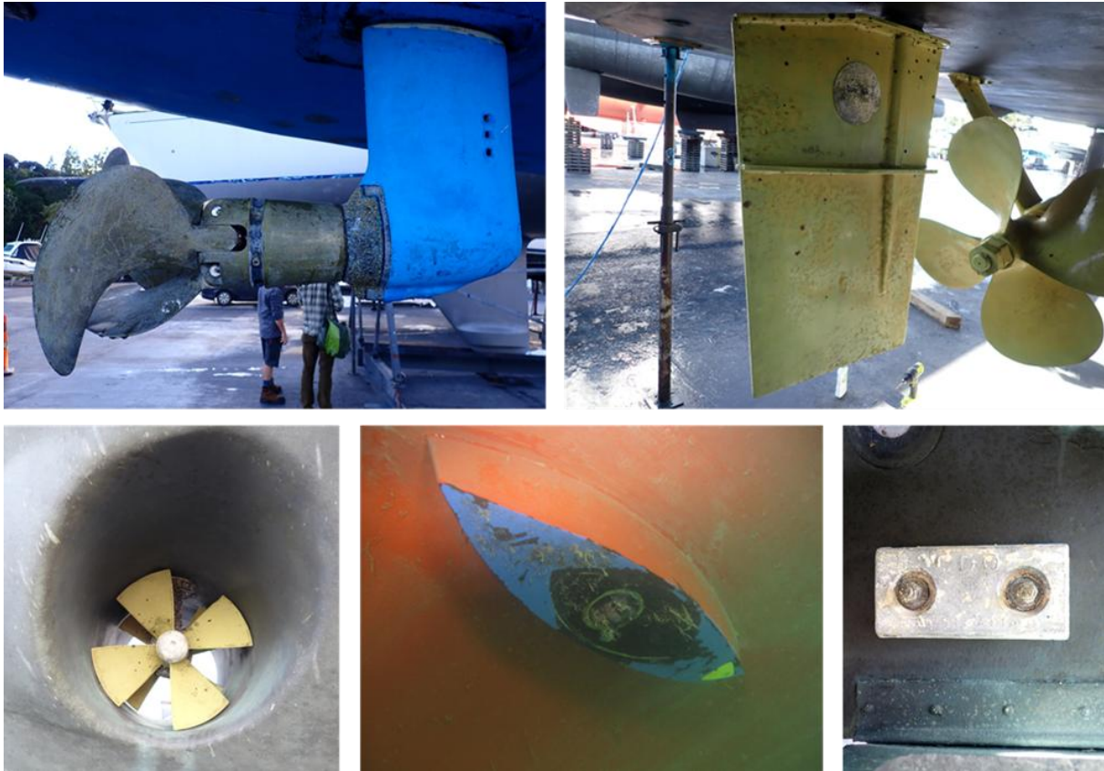
Figure 12. Examples of niche areas measured from boats on hard stand. Clockwise from top left: propeller, shaft, and skeg; rudder; anode; transducer; thruster tunnel and propeller. For each niche area, basic measurements of length, breadth and height were taken, plus surface dimensions of cylinder and circular areas used for calculating surface areas.
