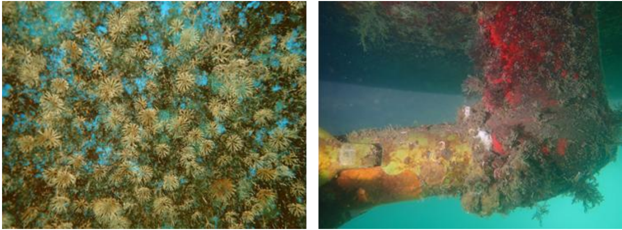
Figure 9. Examples of LOF 5 on a vessel's hull and propeller shaft / strut.
