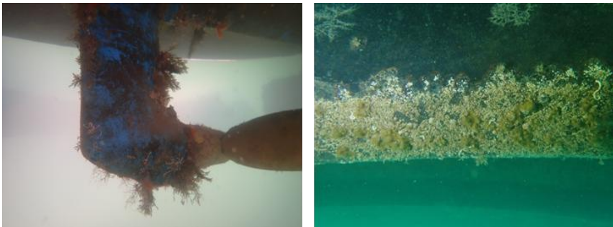
Figure 8. Examples of LOF 4 on a vessel's running gear and keel.
