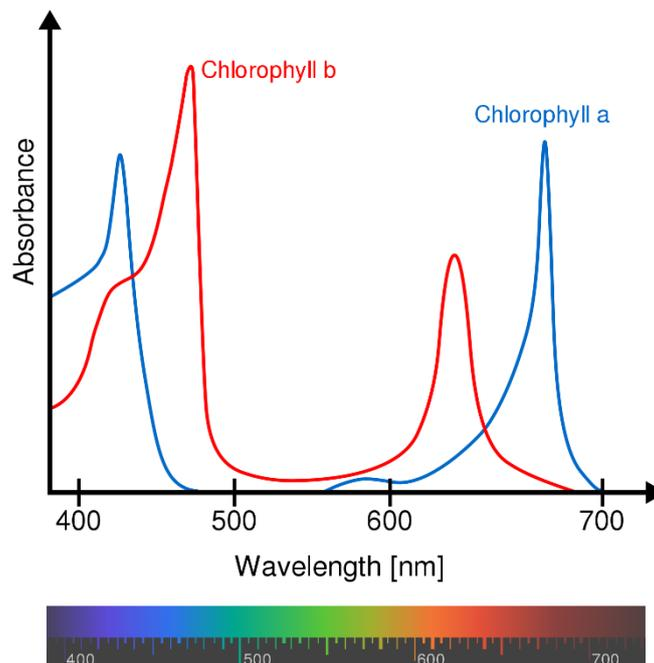
Figure 2. Absorbance spectra of free chlorophyll-a (blue) and chlorophyll-b (red) in a solvent. The action spectra of chlorophyll molecules are slightly modified *in vivo* depending on specific pigment–protein interactions. Source: 'Chlorophyll ab spectra' by Daniele Pugliesi, licensed under CC BY-SA 3.0.
