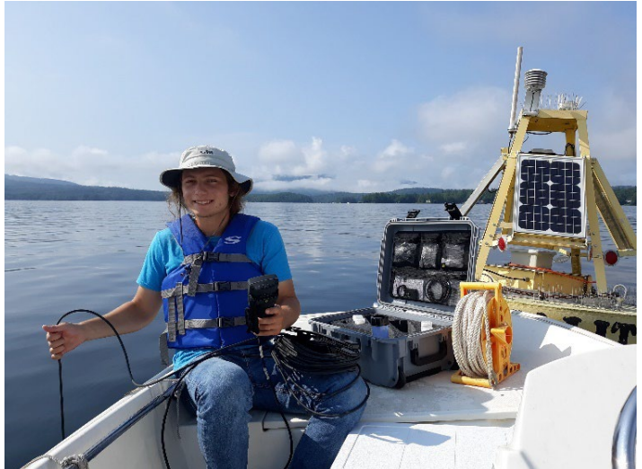
Profiling with a YSI ProDSS at a lake buoy with an EXO sonde at 2 m depth [Whitney Woelmer, University of Waikato].
