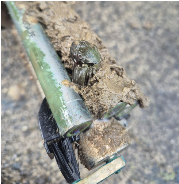
Figure 10. Examples of fouling on wiped sensors. (A) PME miniDOT (top) with battery operated miniWIPER after an urban stream deployment. (B) In-Situ Aqua TROLL after deployment in Te Waihora, a coastal lagoon. (C) A wiped In-Situ RDO Pro-X sensor after deployment in Te Waihora, a coastal lagoon. (D) In-Situ RDO Pro-X with ZebraTech Hydro-Wiper after deployment near the mouth of Te Waihora, a coastal lagoon. (E) Heavily fouled sensor bodies on an YSI EXO sonde retrieved from an estuary. (F) Heavily fouled YSI EXO sonde retrieved from Wainono, a coastal lagoon.
