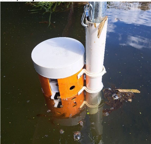
PME miniDOT and miniWIPER installed in Horseshoe Lagoon, Canterbury [Julie Grant, ECan].
