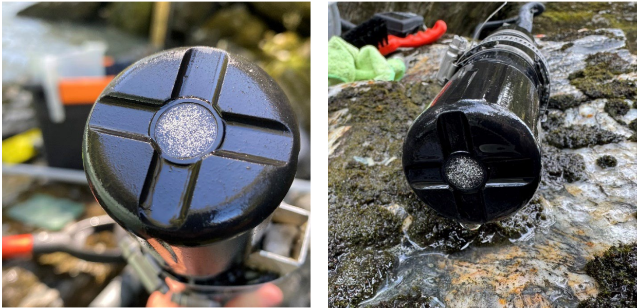
Figure 15. Sensor foil damage on an In-Situ RDO Pro-X after abrasion by coarse sediment transported during a high flow event on the Rees River (see back cover) [Emily Olson, ORC].
