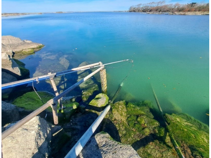
DO sensor verification check on the Opihi lagoon [Julie Grant, ECan].
