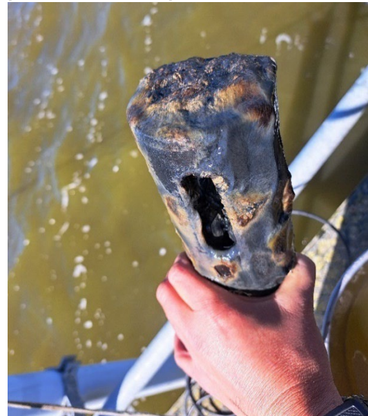
Figure 10. Examples of fouling on wiped sensors. (A) PME miniDOT (top) with battery operated miniWIPER after an urban stream deployment. (B) In-Situ Aqua TROLL after deployment in Te Waihora, a coastal lagoon. (C) A wiped In-Situ RDO Pro-X sensor after deployment in Te Waihora, a coastal lagoon. (D) In-Situ RDO Pro-X with ZebraTech Hydro-Wiper after deployment near the mouth of Te Waihora, a coastal lagoon. (E) Heavily fouled sensor bodies on an YSI EXO sonde retrieved from an estuary. (F) Heavily fouled YSI EXO sonde retrieved from Wainono, a coastal lagoon.
