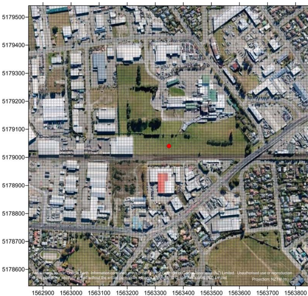
Figure 3: Modelling domain and gridded receptor spacing for the diesel-fired generator. Axes are in metres, in NZTM coordinates.
