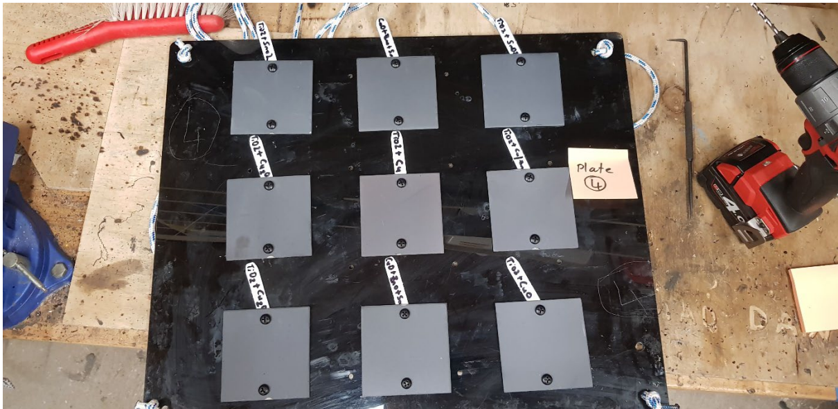
Figure A1.1. Backing plate with replicate plates attached. Image: P. Cahill, Cawthron.
