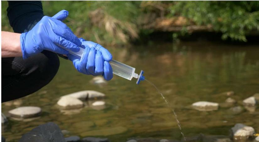
**Figure 7-2: Active eDNA sampling using the Wilderlab barrel syringe and filter.** Image sourced from Wilderlab.co.nz.
