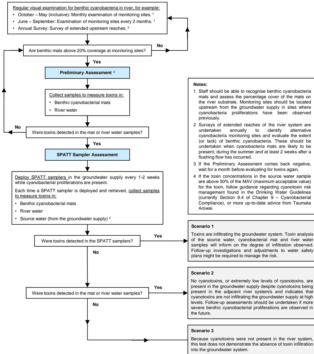
Decision-making framework for evaluating cyanotoxin risk in groundwater supplies with likely connectivity to surface waters containing potentially toxic benthic cyanobacteria.
