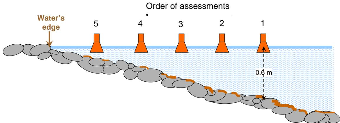
Schematic of transect cross-section showing arrangement of sampling points (not to scale). Notes: Assessment 1 will cover a greater area than Assessment 5 because of the greater water depth. However, this will be the case at all sites, and therefore assessments should be comparable. Image credit: C. Kilroy, NIWA. Source: New Zealand guidelines for cyanobacteria in recreational fresh waters.
