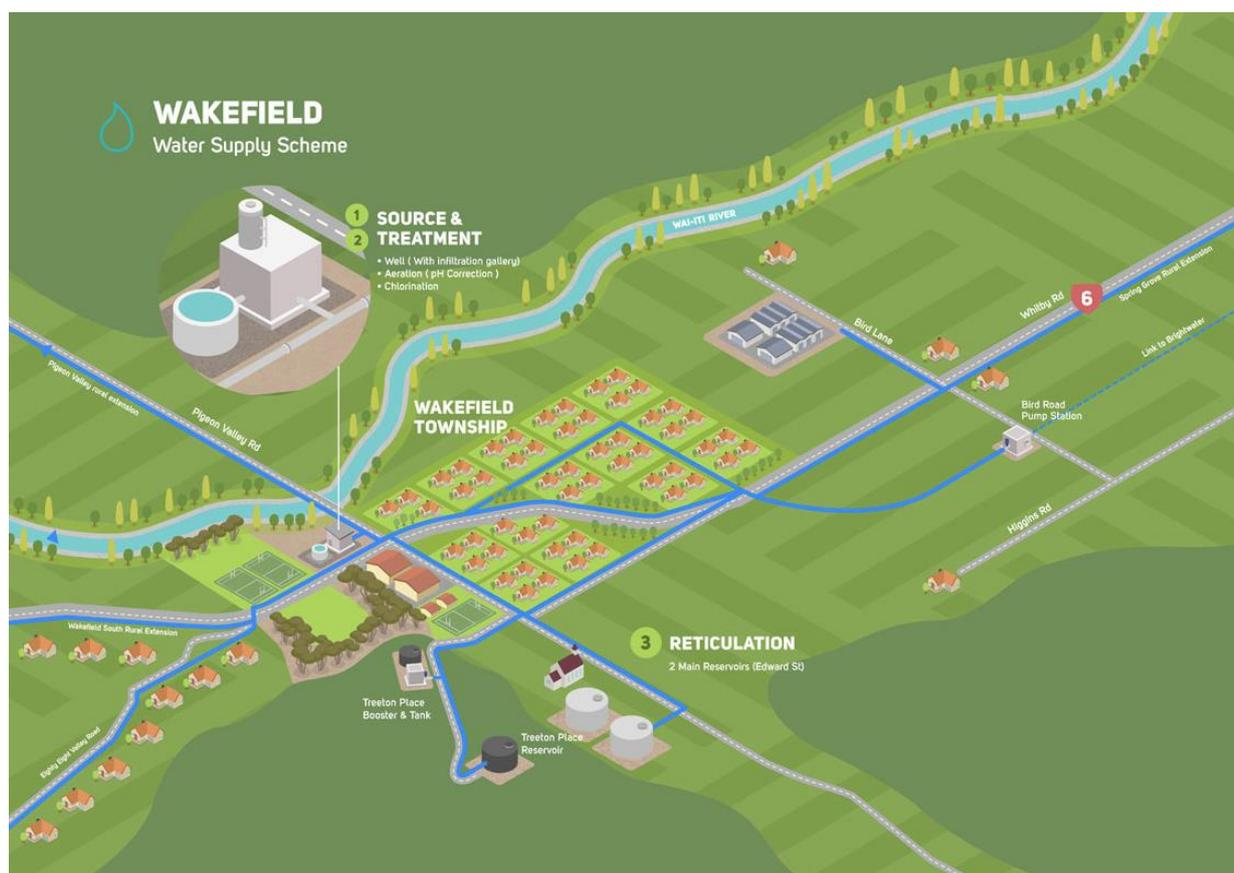
Figure 2. Schematic of the Wakefield water supply, which draws source water from the Wai-iti River through an infiltration gallery and into a shallow well (TDC 2024a; note that this schematic may no longer be current).
