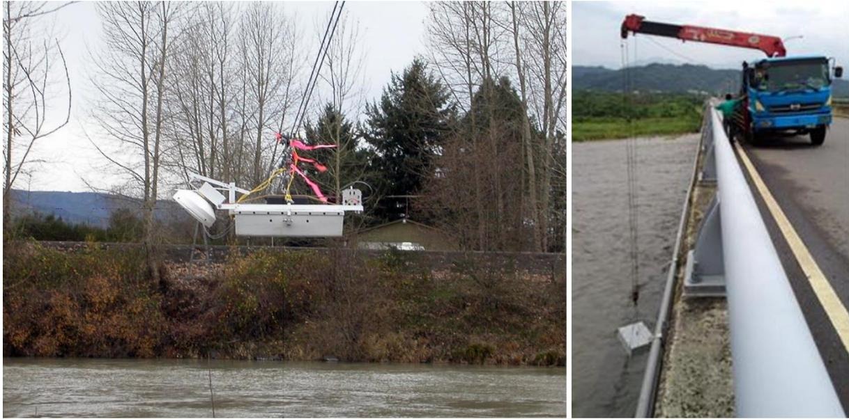
**Figure 3-3:** Left: Deployment of a GPR antenna and doppler radar system on a cableway by Costa et al. (2006). Right: Deployment of a GPR antenna from a bridge by Hong et al. (2017).
