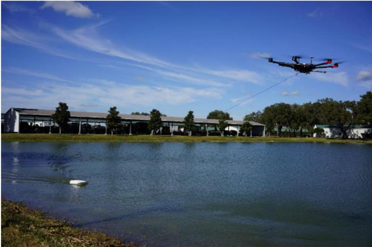
**Figure 3-10: Bathy-Drone depth sounder system, towed by a DJI M600 drone.** Image from Diaz et al. (2022).
