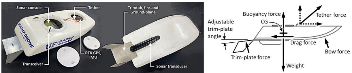
**Figure 3-11: Bathy-Drone components and forces.** Image from Diaz et al. (2022).
