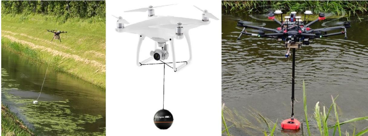
**Figure 3-9: Left: Tethered sonar towed by DJI M600 drone. Centre: Tethered sonar towed by DJI Phantom 4 drone. Right: Rigidly attached depth sounder on DJI M600 drone.** Image credits (left to right) are: Bandini et al. (2018), Koutalakis and Zaimis (2022), Coppo Frias et al. (2024).
