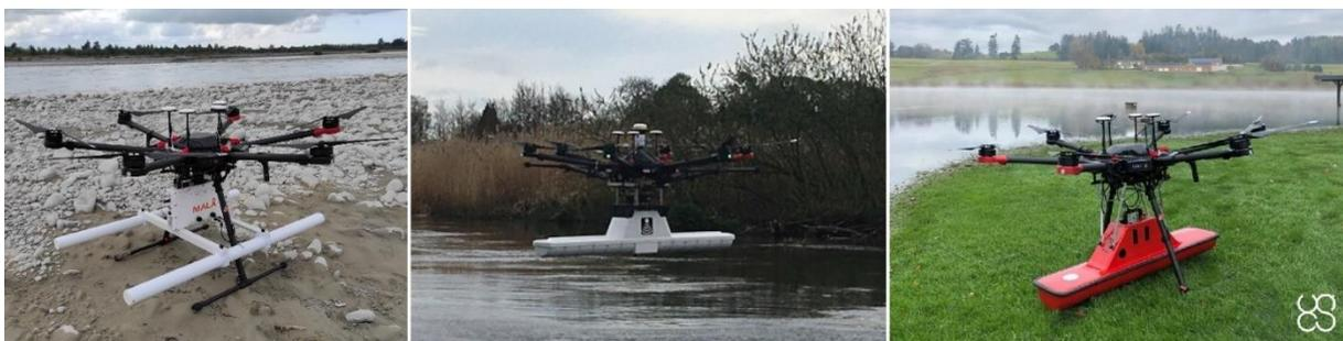
**Figure 3-4:** Lightweight aerial GPR antennas on DJI M600 drones. Left: MALÅ GeoDrone80 (Biggs 2022). Centre: Geoscanners Gekko-80 (Bandini et al. 2023). Right: RadarTeam Cobra SE-150 (Image from: <https://shop.sphengineering.com/products/cobra-plug-in-gpr>).
