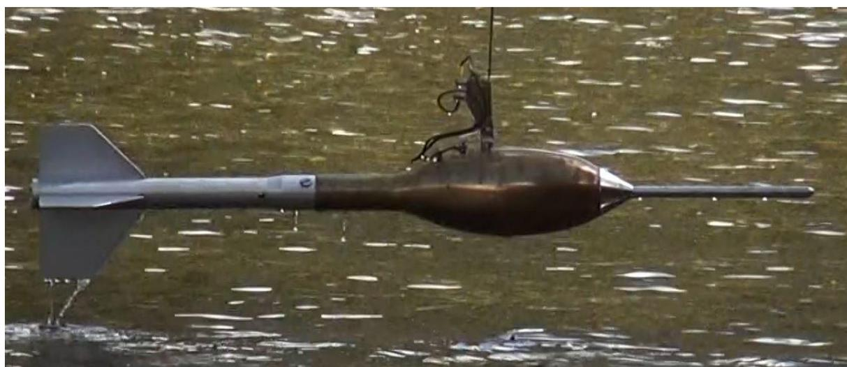
**Figure 2-3: Pressure Operated Electronic Meter (POEM) for measuring velocities and depth from bridges and cableways.**
