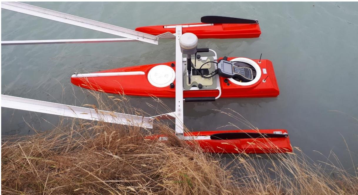
**Figure 2-4: Tritech PA500 depth sounder connected to Trimble R10 RTK GPS Rover and mounted on an ADCP boat hull.**
