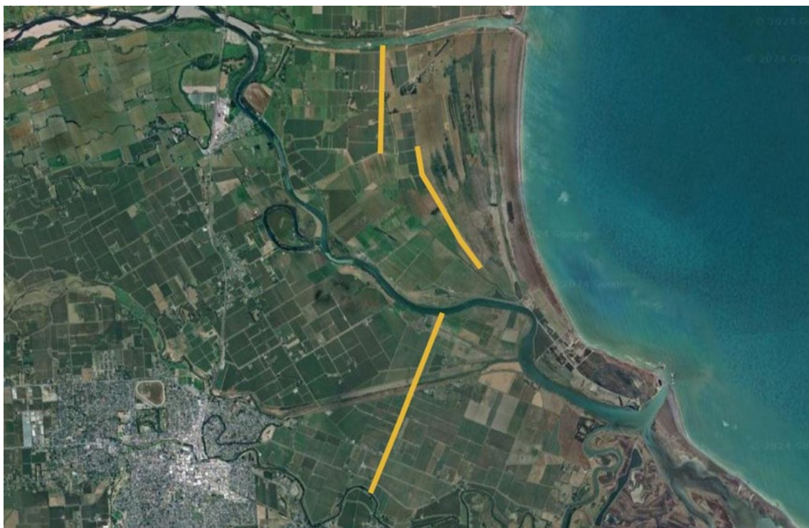
Figure 4.4 Proposed seismic lines across the coastal Wairau Plain. Total length 10 km.
