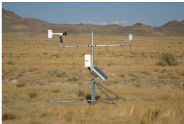
Figure 5. Automatic mobile weather station, with sensors, data logger and solar battery.
