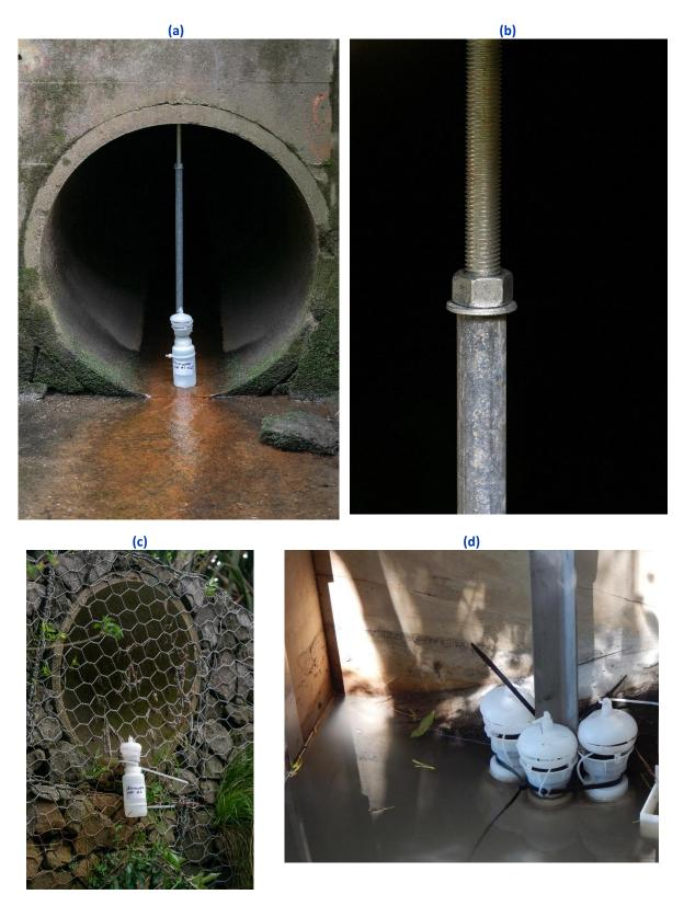
Figure A-6: Bottles mounted (a) with an extendable threaded rod; (b) close up of the threaded rod; (c) using existing steel mesh on a stormwater outlet; and (d) to a piece of steel angle, dynabolted to the side of a stormwater outlet wingwall.
