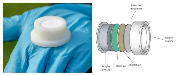
**Figure 3-3:** DGT devices for water sampling (left) and schematic of key components of DGTs (right). [Photo: Stuart Mackay. Schematic: Knutsson et al. (2014)]
