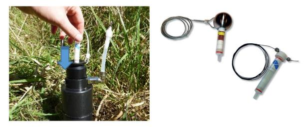
Figure 5-7: Mounting options for Sorbicells for monitoring of stream water using WW-50 (left) and stormwater using steel ball or plastic mounting (right). [Sorbisense Limited]
