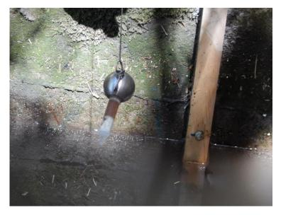
Figure 5-8: Sorbicell deployed in steel ball at the Akatea Road stormwater site.
