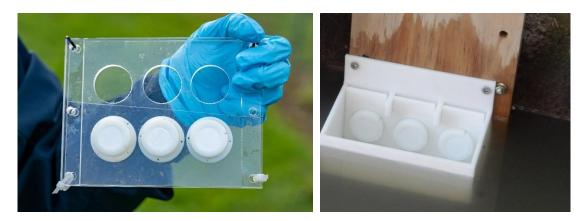
Figure 5-4: Holders for DGTs for monitoring of stream water (left) and stormwater (right).
