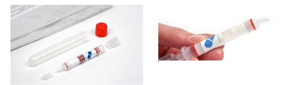
Figure 5-9: SorbiCell sampler, protective cap and transportation tube with red cap (left). Pre-wetting of SorbiCell using syringe with Milli-Q water (right).
