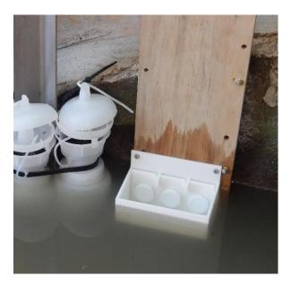
Figure B-4: DGT trough holder mounted to (a) extendable pipe inside a stormwater pipe for a temporary installation and (b) timber bolted to stormwater outlet wing-wall for a more permanent deployment location.
