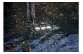
Figure B-5: Deployment steps showing (a) DGTs contained within acrylic plate (b) with temperature recorder attached and (c) and plate attached to waratah.
