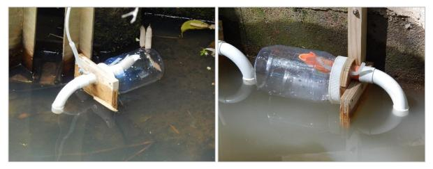
Figure 5-5: Modified siphon sampler bottles mounted to frame in Whau Creek (left) and at Akatea Road stormwater site (right).
