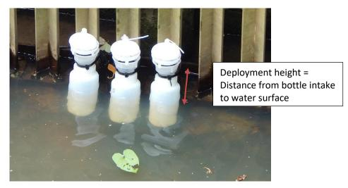
Figure A-3: Deployment in a stream showing the deployment height.
