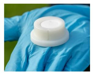
Figure B-1: DGT device for sampling water. Photo credit Stuart Mackay, NIWA.
