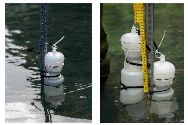
Figure A-5: Stormwater sampler bottle attached to a waratah stake in a stream, deployed as individual or multiple bottles at different heights.
