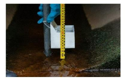
Figure B-6: Installing trough on an adjustable pipe and measuring deployment height.
