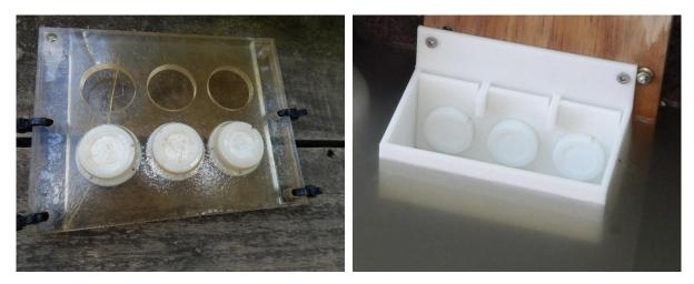
Figure B-3: Housings for DGTs for monitoring of stream water (a) and stormwater (b).
