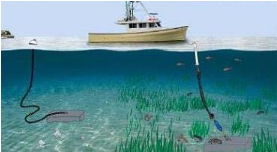
Figure 4. Traditional (left) versus elastic (right) mooring ropes. Source: http://www.atlanticfishhabitat.org/Documents/21981ProtectingEelgrassHabitat-2_000.pdf , accessed 25 October 2017.
