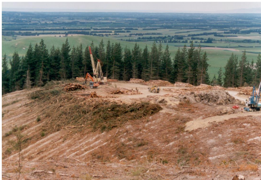
Figure 7: A typical steep terrain cable logging harvesting operation showing trees being extracted and processed into logs on the landing, whereby the harvest residue is discarded off the landing edge.
