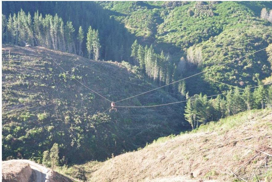
Figure 15: Cable logging across a gully system – if not enough deflection is available then extracting stems from the back face will sweep the logging slash into the gully system.
