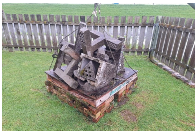
Figure 3.2. Various designs were made, some registered by Design Marks and called Bio Links, Cray Haven and Sea Drops. They were deployed down a fused rope in an effort to aggregate the materials on the seabed.
