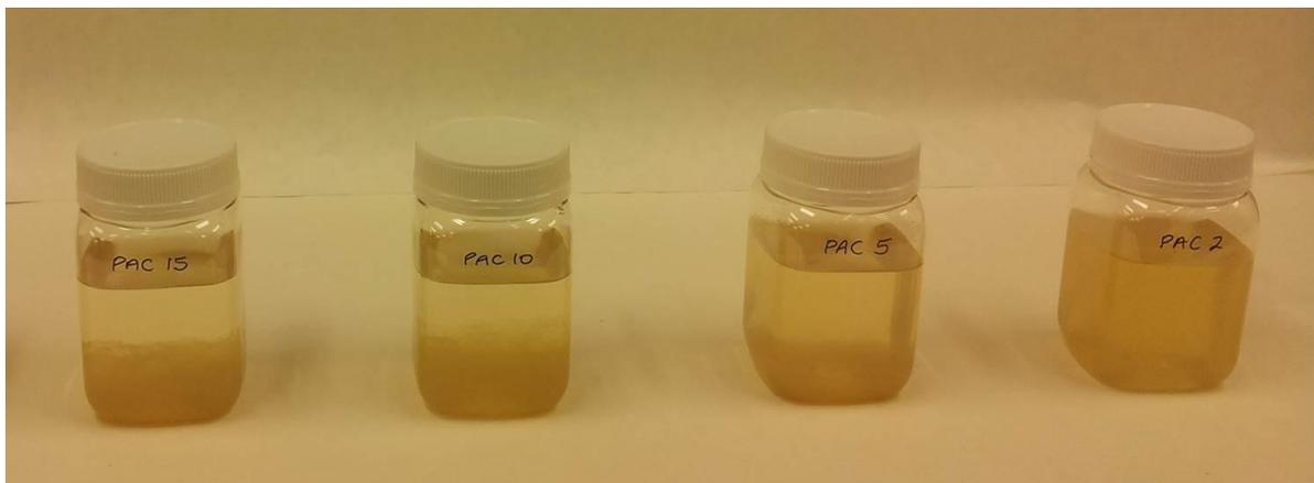
Figure 12 Testing efficacy of a flocculant (PAC; polyaluminium chloride) at different concentrations (2 – 15 mg L<sup>-1</sup>) for potential application in Lake Oranga (University of Waikato).
