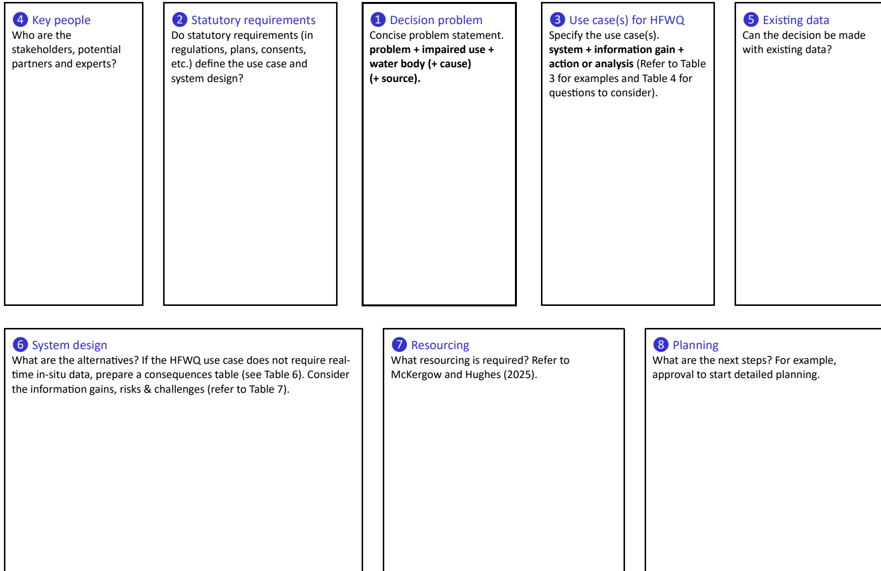
Figure 6. Framework to support initial planning to design and justify a HFWQ monitoring system to support decision-making (adapted from Timmerman et al. 2022). The decision problem is deliberately positioned in the centre of the framework to ensure it remains in focus.
