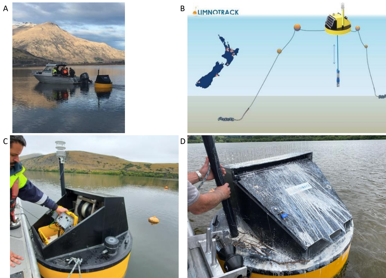
Figure 4. Lake Hayes monitoring buoy installation in July 2019. (A) Buoy being towed to the site [ORC]. (B) Diagram of the mooring [provided to ORC by Limnotrack]. (C) Buoy installed [ORC]. (D) Fouled buoy despite bird spikes [ORC].
