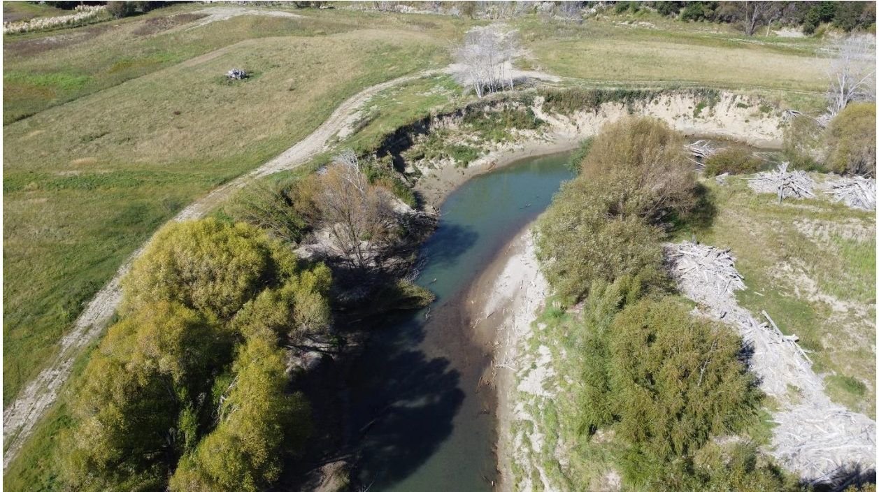
Figure 29. Sparsely treed outer bends showed more toe erosion and slumping.
