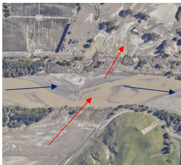
Figure A11. Directional effect of Ebbetts floodplain return flows & Dartmoor stopbank breach flows.
