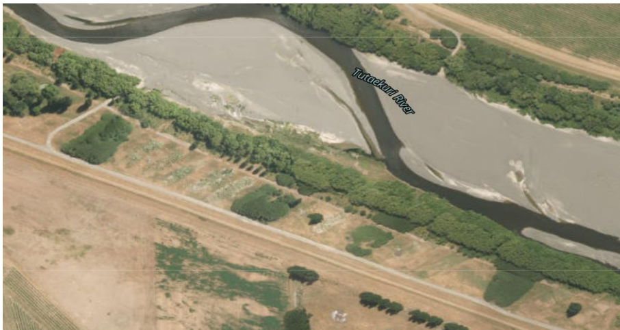
Figure A13. Pre-cyclone berm with buffer zone & chevron planting.
